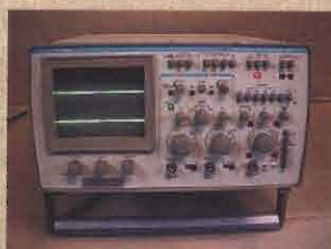
DIGITAL STORAGE OSCILLOSCOPE GOULD type 4030
